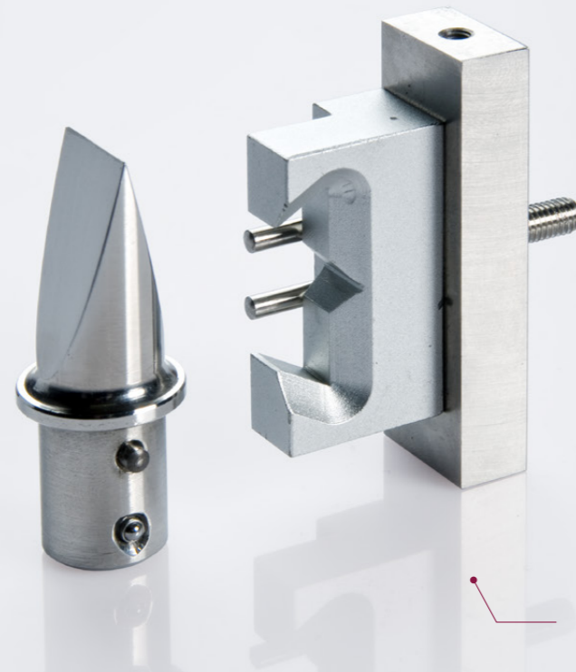
Evaluates the tensile strength of oblongs utilizing specialized inserts
