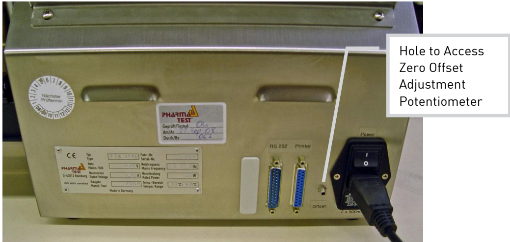
Figure 21: Hole to Access Zero Offset Adjustment Potentiometer
