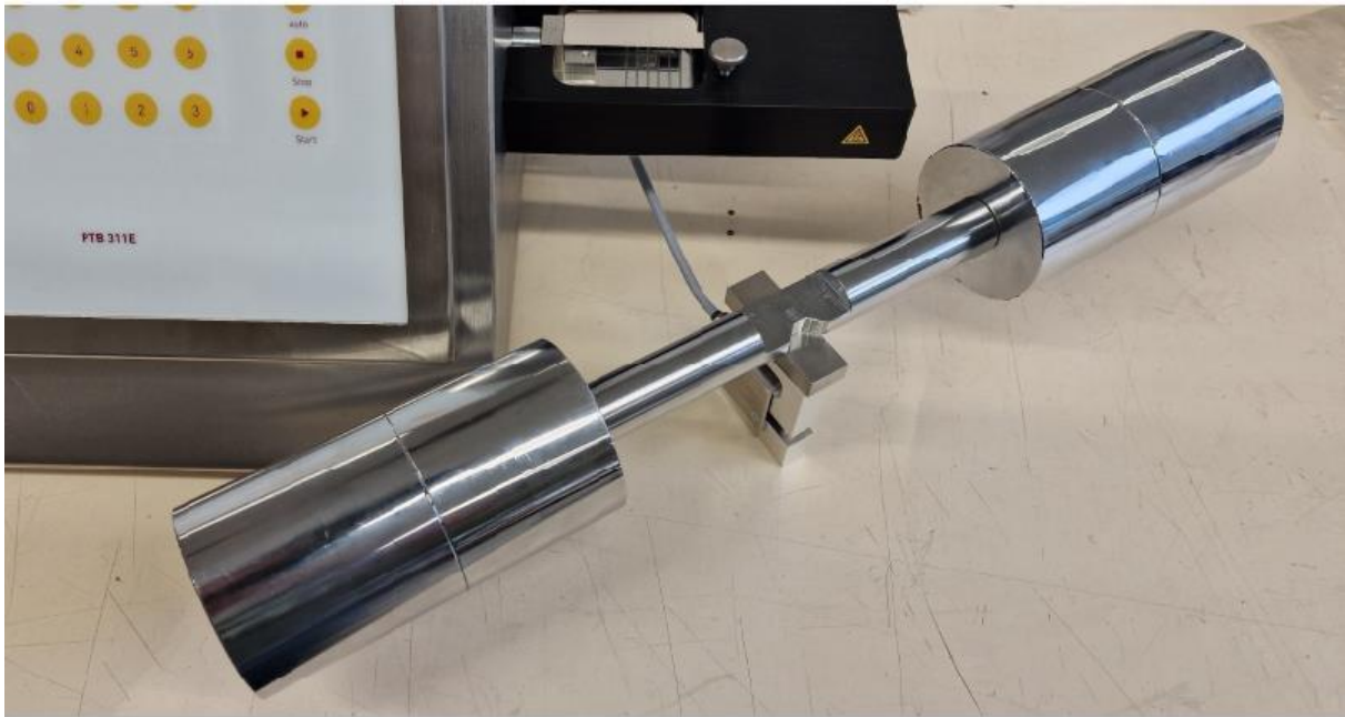
Figure 22: 10kg Reference Weight On Top Of Load Cell
