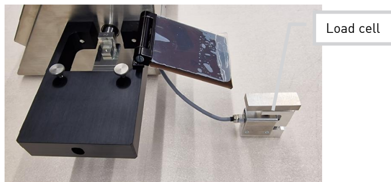
Figure 20: Load cell in upright position - ready for adjustment and calibration
