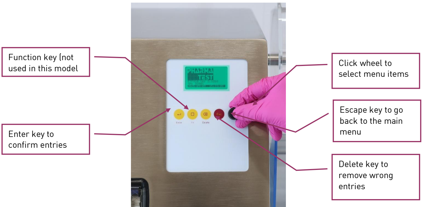
Figure 4: Control Panel of the Instrument
