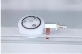
The water bath cover is constructed from PVC, offering dimensional stability, resistance to dissolution media, and ease of cleaning. Dissolution vessels are inserted directly into the water bath cover and secured using centering rings equipped with a 3-way bayonet catch mechanism.
