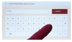
All instrument interactions are carried out via a capacitive touchscreen interface, engineered to remain highly responsive even when operated with laboratory gloves. This design not only enhances user convenience but also supports strict hygiene standards in laboratory environments.
