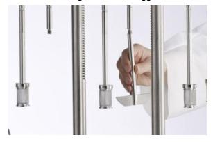
PTWS 1230 uses the Pharma Test MonoShaft design with a main shaft and interchangeable tool heads. The shaft stays fixed in the instrument, keeping tool clearance consistent after initial installation. Each stirrer can be manually lifted for easy vessel access.
