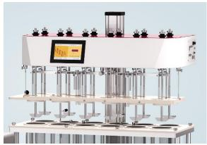
The Plexiglas water bath features a quickconnector system ensuring secure, leak-free attachment of the heater module to the water bath.
