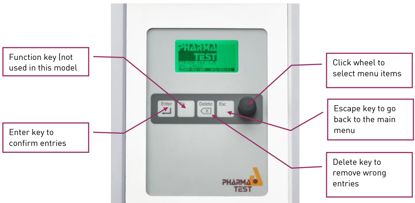
Figure 4: Control Panel of the Instrument
