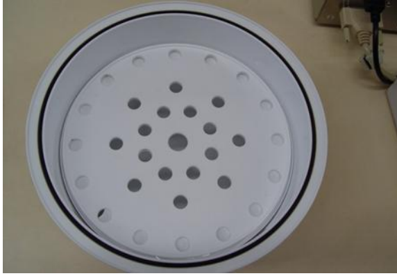
Figure 7: Sealing ring inserted properly
