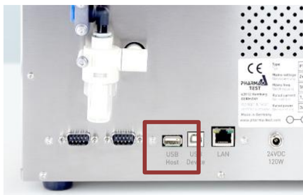
Figure 18: Port for USB flash drive
