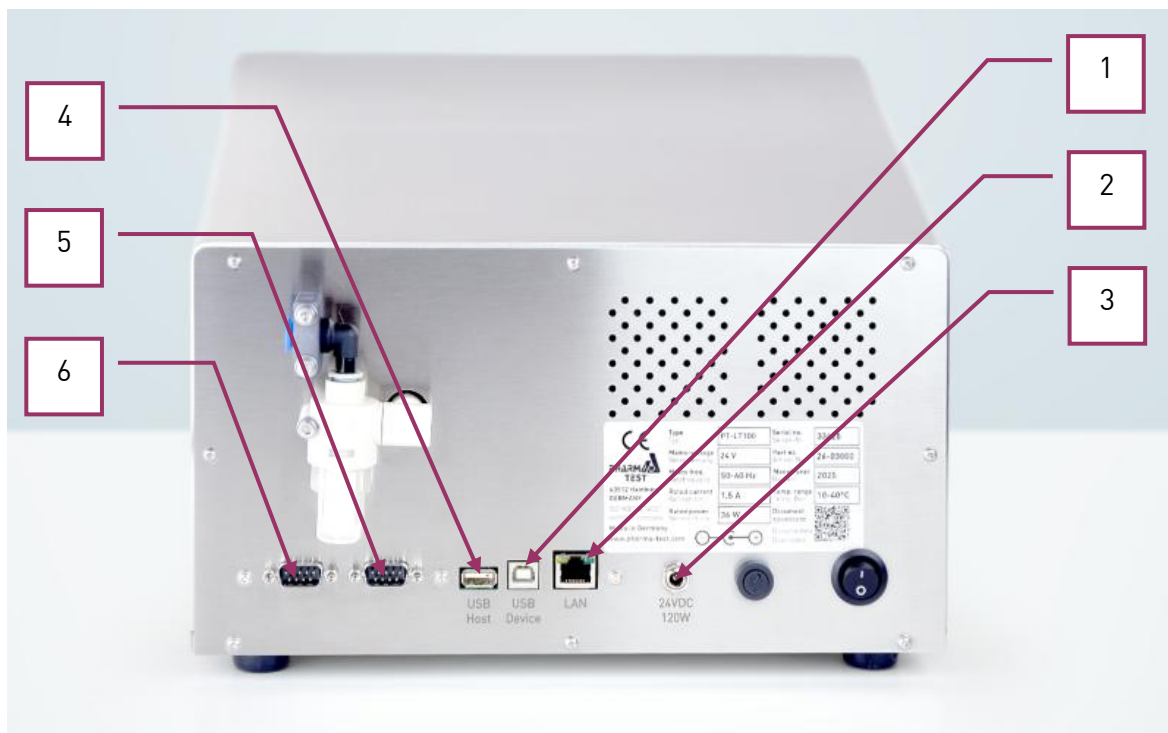
Figure 17: Instrument Overview – Interfaces
