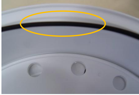
Figure 8: Sealing ring not OK
