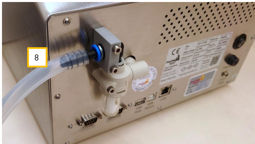
Figure 11: Connecting tube to vacuum inlet
