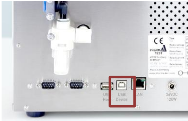
Figure 21: Port for PC connection
