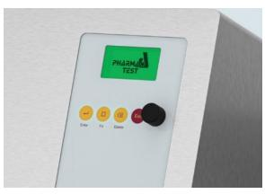
PT-LT100 is operated by using a click wheel to navigate menus on the LCD screen and by functional keys to shortcut frequent operations. The display is backlit in changing colors that show the instrument status in a familiar traffic light system (green, yellow, red). Navigating the menu is quick and simple. The color-changing display makes it easy for the user to see when his input is required to proceed.
