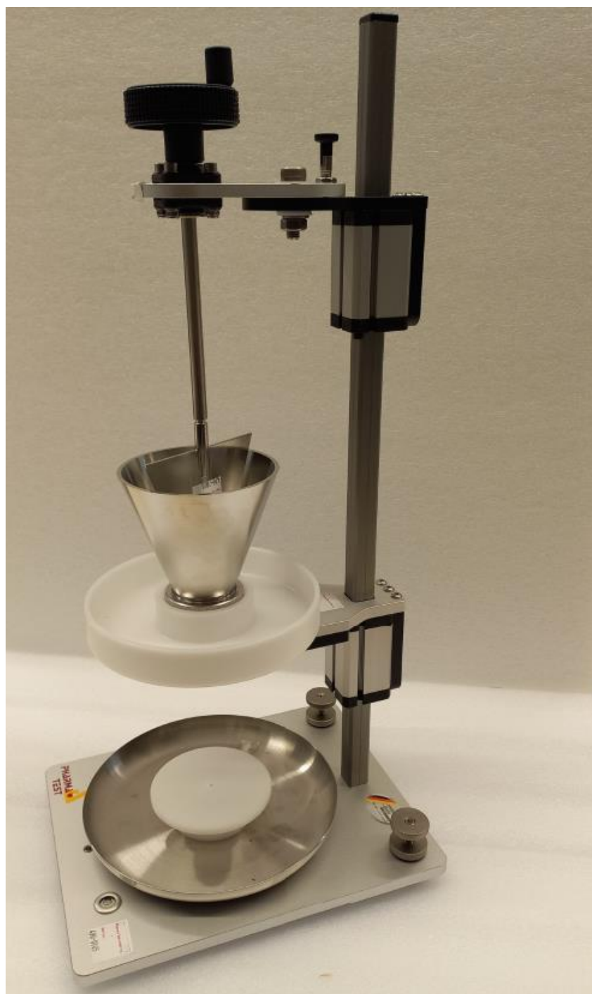
Figure 1: Overview PTG-M100 in the Configuration for Flow Measurement, with Manual Stirrer
