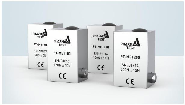
Not replacing periodic calibration, the PT-MET set performs as a daily verification, much like a balance is checked at the start of each day and can be recorded in the instrument's logbook. The PT-MET mechanical tablets come as a set of four or can be purchased individually. They come with a certificate of calibration, operating instructions and can be returned to us for re-calibration.
