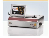
PTB 420 is an automated, dual test mode instrument to determine the diameter, thickness and hardness of tablets. Thickness is detected by an optical system.
