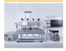
The new 8-station DFC-820SP auto-sampling dissolution system is fully USP, EP and JP compliant. The long-term and reliable operation includes well engineered, stable mechanics.
