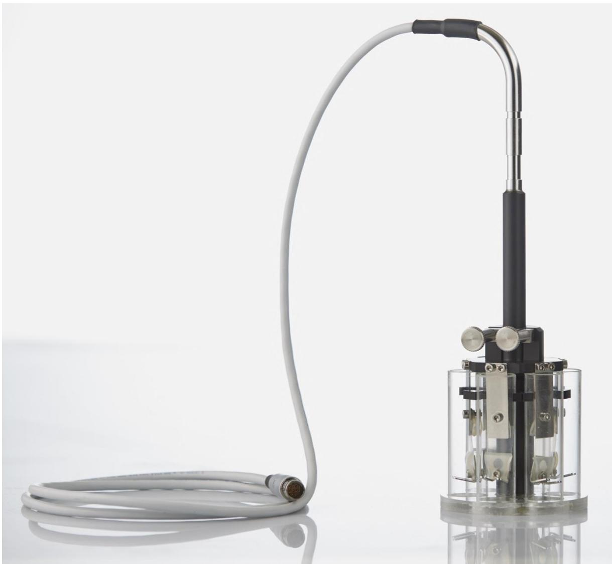
The PT-ODF test basket add-on for the PTZ AUTO EZ tablet disintegration testing instruments closes this gap by offering a simple and affordable device to reliably test the disintegration times of films. The PT-ODF basket can be used with any existing Pharma Test PTZ AUTO EZ instrument without any need
