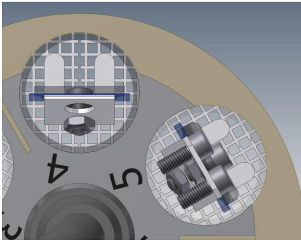
The weights hit the split metal sieve of the PT-MKT basket and close an electrical circuit. The instrument detects this and automatically logs the disintegration time.
