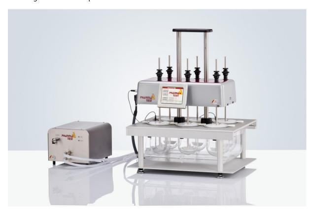
If certain operational parameters form a regular feature of the daily routine, then these can be incorporated into a test method for faster set up. These parameters can be tool speed, target bath temperature, sampling time points and so on. The test method memory capacity is almost limitless.
