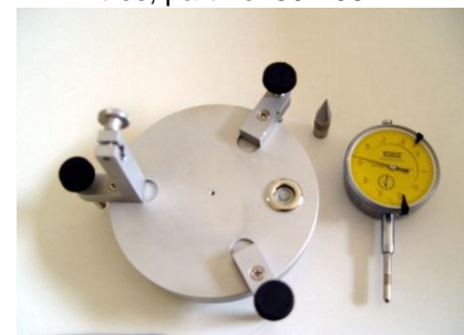
SWT2 shaft wobble and centricity tester, for PTWS part no. 30-31210, for PT-DT70 part no. 30-31220
